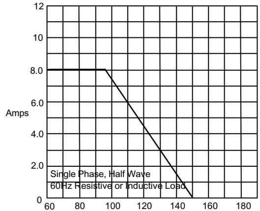
Average Forward Rectified Current - Amperes versus
