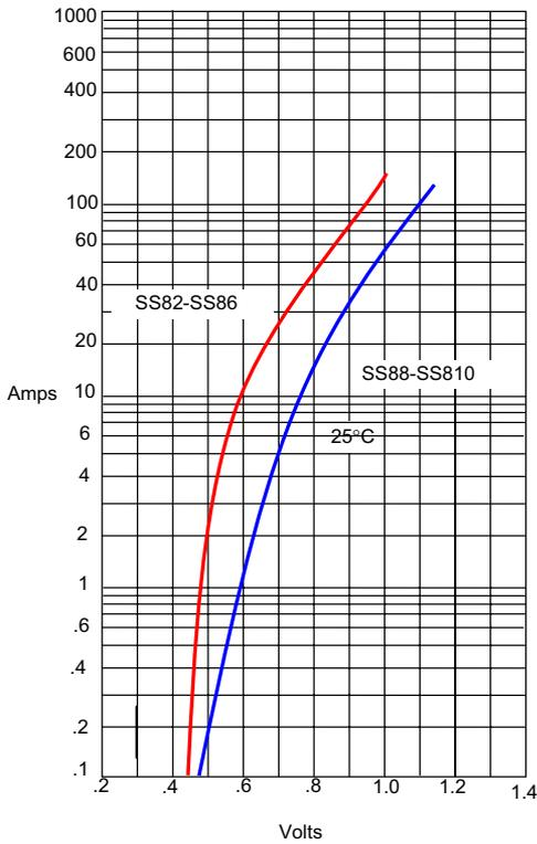
Instantaneous Forward Current - Amperes versus
