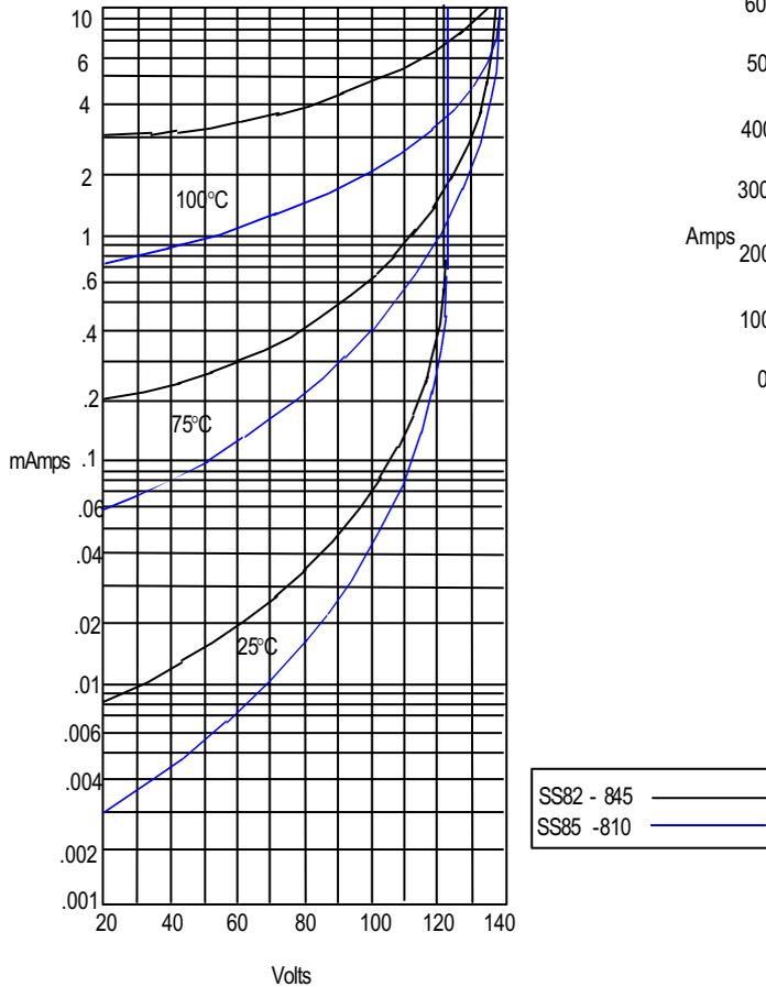
Instantaneous Reverse Leakage Current - MicroAmperes versus
