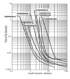
◆ Time to Trip curves represent typical performance of a device in a simulated application environment. Actual performance in specific customer applications may differ from these values due to the influence of other variables.
