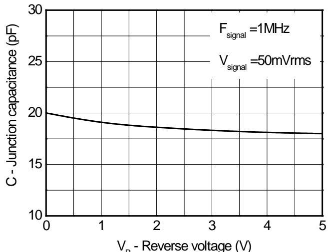
Capacitance vs. Reveres voltage
