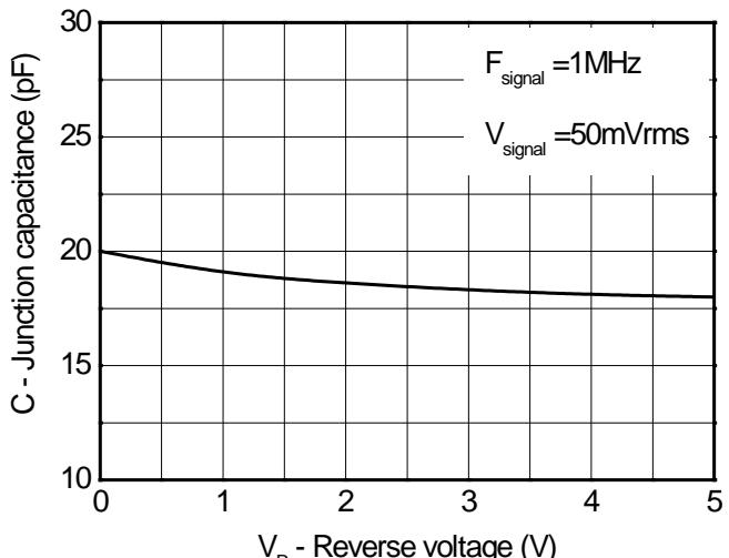
**Capacitance vs. Reveres voltage**
